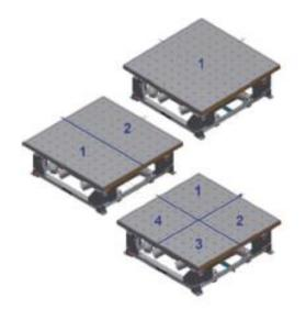
HALT and HASS testing more controllable and consistent. Each zone can also be set to a different Grms level or Multi-Zone Control can be turned off to control the entire table to one Grms level.
