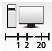
A serial bus interface can be used to connect appliances to an external monitoring system. If there is no monitoring system that can be connected via the interface available, an interface converter retrofitting kit (which connects with a PC or laptop) can be obtained as an optional accessory. The bus interface can be used to serially connect and network up to 20 appliances. Temperature and alarm details can be documented and archived using Temperature Monitoring software.
